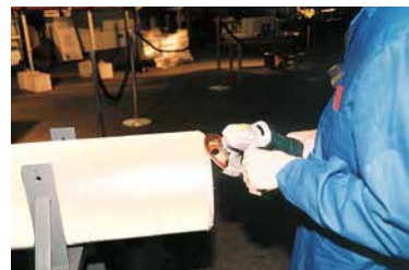
Bevelling using a rasp disc
